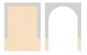
Try to avoid supporting the functional areas of the part. If one side of the part is supposed to slide in or fit with another part, it is recommended not to place supports on that side to prevent scarring and additional post-processing. MAGS AI allows marking these key areas, and automatically orientates and supports the part accordingly.
